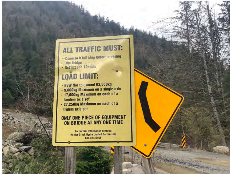
Load Rating Sign
